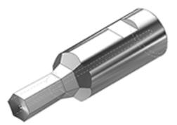
Polygon Solutions' 1/2" shank hexagon rotary broaches are precision ground with a tolerance of +0/-.0005. Each nominal size conforms to the industry standard – ANSI B18.3 2003. All 1/2" shank hex rotary broach tools include a pressure relief vent hole that allows air and fluid to freely escape during the rotary broaching process to reduce wear on your machine and extend rotary broach tool life.
